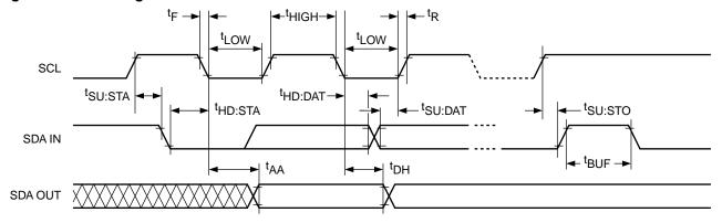
Figure 2. Write Cycle Timing
